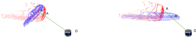
Fig. 2: Example of the point modeling and plane modeling method. The blue points are intra-predicted result using point model or plane model. The residual of point A is OA - OA' .
