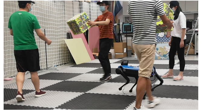
Fig. 7: Real-world experiment in the “box-relay” scenario. The robot safely moves through the crowd which has complex motion patterns without introducing apparent disturbances to the humans.
